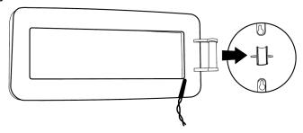
Unroll the **FM** wire antenna and stretch it out. This antenna is permanently attached to the back of the radio. Position this antenna for best reception of your favorite FM station.
